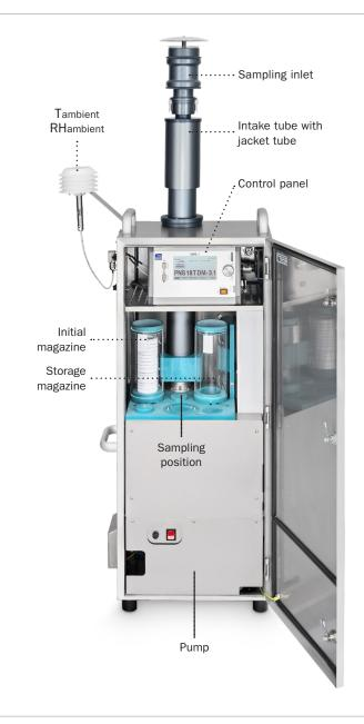
The volumetric flow rate is measured with an orifice plate and is electronically adjusted with an accuracy of  $\leq 2 \%$ deviation. The ambient climatic conditions are continuously monitored by temperature and humidity sensors. The optional Peltier cooler ensures that the sampled filter storage temperature in the unit does not exceed 23 °C.
