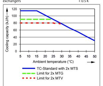
Note: The limit curves for the heat exchangers exchanger PTG, PTV or MTV apply to a dew point of 40 °C.
